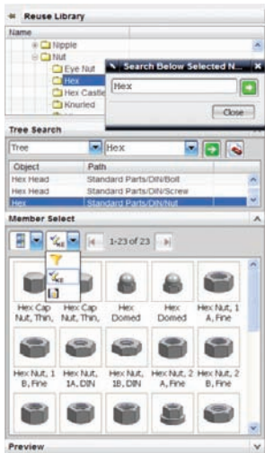
NX Reuse Library provides quick access to re-usable design data throughout the design process
